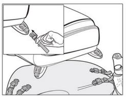
Now fasten the male buckles on both strap 'A' & 'B' into the female buckles on the tank bag and adjust to fit snug. When seated on the motorcycle, make sure you can freely operate all the controls with the tank bag in
