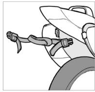
Depending on your bike's configuration, you may have to connect the two bags together with the side straps as shown. Position straps under the fender or licence plate bracket. Do not overtighten. Check the bags from the rear of bike to make sure they are not analed in or out. Bags should be as vertical as possible.
