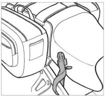
Using the strap with buckle on one side and loop on the opposite side, hook it or loop it around the frame, foot peg or secure body part and then back into the clip on the bag. You can also pass the buckle through the loop creating a noose to attach it around the frame or secure body part.
