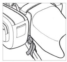
Re-attach strap to bag and adjust to fit. This strap does not need to be overtightened as the side straps mainly hold the bags against the bike only and when installed correctly, do not come under heavy load.
