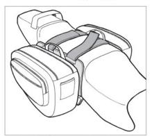
Connect Velcro® straps on each bag together as shown and position over, or if your bike allows, under the seat. Adjust these straps to determine the height of the bags. Further adjustment may be necessary once bags are loaded to ensure they do not come into contact with your exhaust (see diagram below) or moving bike part. For wider vehicles and seats, Velcro® extensions straps can be ordered from our website.
