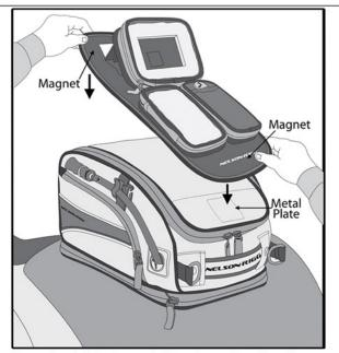
To convert your tank bag from map to GPS ready, you will need to purchase our CL-GPS-MG Journey GPS Mate. First, make sure that the clear map pocket and bottom of the GPS Mate are free from any dust dirt or road grime. Position the GPS Mate on top of the map pocket on your CL-2015 tank bag aligning the magnets in the GPS Mate to the metal plates sewn inside the front of the lid and back of bag. The CL-GPS can also be used by itself on any metal tank as a GPS and phone holder.
