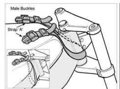
Using Strap 'A' with 2 male buckles on either end, connect one side to a female buckle on the front of tank bag. Loop opposite side around the frame or steering head behind the triple clamp making sure the strap is not pinched by the steering stops or displacing control cable or hoses. Adjust the strap length so the clips lay on the front of the fuel tank just behind the triple clamp. Clip remaining male buckle into open female buckle on tank bag.
