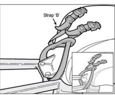
Using Strap 'B' remove or raise the seat of your bike and either pass one of the buckles around the frame tubes or rear fuel tank or pass the loop in the middle of strap 'B' around the frame tubes or rear fuel tank and feed one of the male buckle through the loop securing the strap to your bike. Avoid sharp edges that may damage the nylon strap when it is tight.
