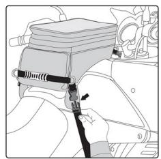
Attach the male buckle to the female on each side of the rear of the bag. A "click" will be heard when the components are pushed together correctly. Tighten straps sufficiently to remove all slack. Final tensioning will be done after front strap is installed. Fold slack ends of straps and secure by passing through elastic webbing loop on each strap.
