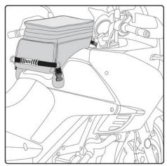
Position bag on tank of the motorcycle making sure bag is centered and free from all moving and hot parts. Always store heavier items in the bottom of the bag for better weight distribution and balance.
