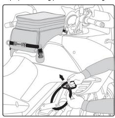
To secure the rear of the bag take the strap with male buckle on one side and loop on the opposite side, pass the loop around a part of the frame or other solid bike part, then push the plastic buckle through the loop creating a noose.
