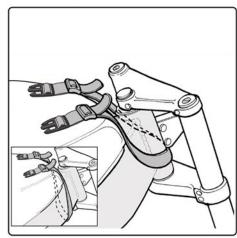
Using the strap with 2 male buckles on either end, connect one side to a female buckle on the front of tank bag. Loop opposite side around the frame or steering head behind the triple clamp making sure the strap is free of steering stops and any cable or hoses. Clip remaining male buckle onto the other female buckle and adjust the strap length.
