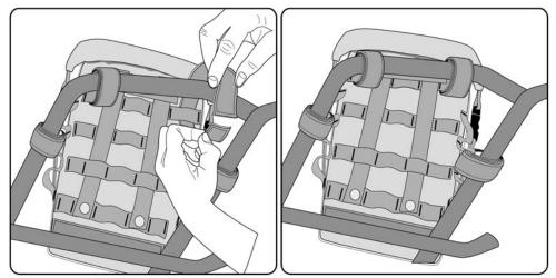
Hold RiggPak up to your mounting location and identify the loops on the back of the bag that line up with the mounting locations. Feed the Hook & Loop straps through the loop on the back of the bag, beginning at the top, wrap the strap around the bar and secure the strap. Repeat on the remaining 4-6 Hook & Loop straps.
