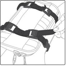
Once in position, pull the strap through the cam buckle until tight. Repeat on all 4 hooks and straps. As an alternative you can attach the bag to the fork tubes to help prevent the bag from sliding down the fender.
