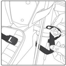
To do so, start by looping the provided straps around the fork tube and under the lower triple clamp making sure you don't pinch any cables or wires. Pass the end of the strap through the loop and pull snug.
