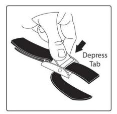
Pass the end of the strap through the cam buckle by pressing down on the aluminum tab and passing the strap through the back of the buckle and pulling tight.
