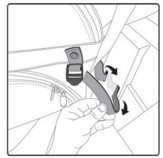
Using one of the lower straps on the side of the bag, attach to secure location or for RZR, pass strap thru the side slot closest to the front of vehicle and loop back thru the next slot and pull excess strap through. Accessing this from the side of the vehicle make this easier.
