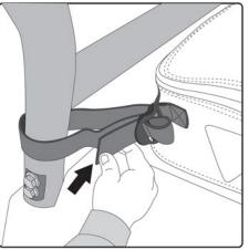
On the end of each side, wrap the 2 straps around the upright roll cage bar and thread back thru the buckle and pull tight.
