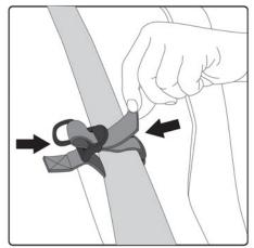
Place the cargo bag in bed of RZR or UTV with door flaps facing the rear of vehicle. Attach the 2 top straps to the cross bar, wrap webbing around the tubing and threading thru the buckle and pull tight.
