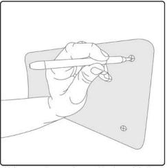
Using a center punch or awl tool, mark in the center of each cross hair making sure the template does not move.
