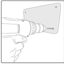
Use a 9mm, Wire size "T" or 23/64" drill bit to drill the holes. Be careful NOT to let the drill go too deep thru the door panel or damage outer skin or internal parts
