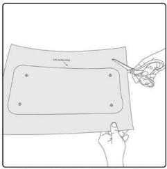
Using the supplied template, cut along lines and tape in the desired location. Always make sure that you do not come into contact with any moving parts or obstructing the normal function of the door.
