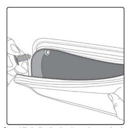
Once drilled, align the door bag or knee pad and insert the provided push pins thru the grommets in the bag and into the door holes.
