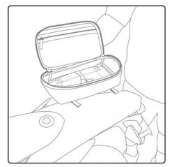
When lining up the bag on your rear fender, always be sure to check under the fender for any wires or cables so they do not get cut or damaged when drilling your mounting holes.
