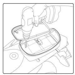
Once you bag is in place on your fender, using a 1/4" bit, drill 4 holes into the plastic bottom your bag and though the fender where you want your mounting points to be.
