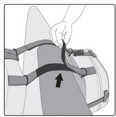
Place Self Fastening straps over seat and level bags. Adjust height of both bags and attach the hook and loop webbing together. Take caution that bag is not on hot or moving parts.
